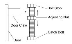
Figure 12 - Catch Bolt and Door Claw Orientation
